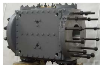
New ACI cast ductile iron, jacketed 150 psig MAWP, 7.0 in. bore, 11.0 in. stroke, third stage cylinder.
