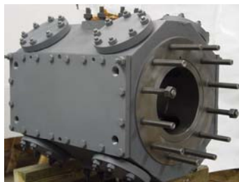
New ACI cast ductile iron, jacketed 150 psig MAWP, 10.0 in. bore, 11.0 in. stroke, second stage cylinder.
